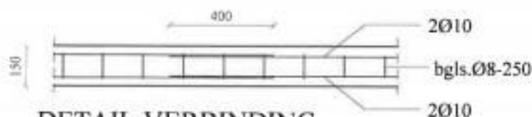
DETAIL VERBINDING OVERLAPPING WAPENING RINGBALK 150MM
